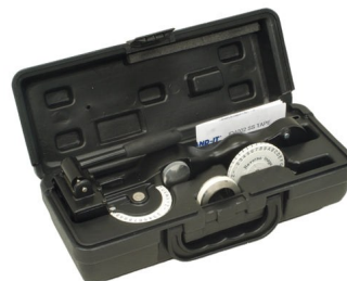
Band-It ID4002 Stainless Steel Embossing Tool
