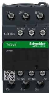
LC1D25F7 TeSys D contactor - 3P(3 NO) - AC-3 - <= 440 V 25 A - 110 V AC coil
