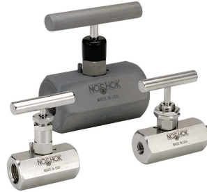
NOS-404-MFS-P1 NOSHOK STD NEEDLE VALVE , HARD SEAT , 1/2" NPT MxF STAINLESS , PTFE PACKING
